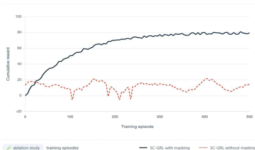
Figure 7. Ablation Study: Training Convergence of SC-GRL with and without Dynamic Action Masking.
